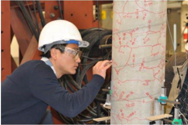
Student Peng Zhang traces cracks in the column during a strength test in UBC Okanagan's Applied Laboratory for Advanced Materials and Structures. Credit: UBC Okanagan
