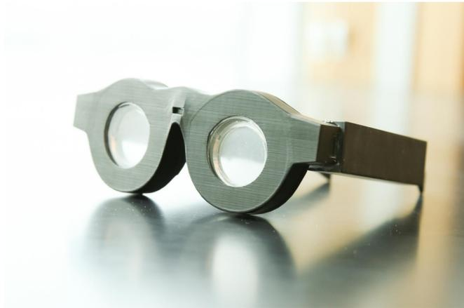
Early prototype of 'smart glasses' with liquid-based lenses that can automatically adjust the focus on what a person is seeing, whether it is far away or close up. The lenses are placed in battery-powered frames that can automatically adjust the focal length of the lenses based on what the wearer is looking at. Researchers expect to have smaller, lighter frames with the technology in as early as three years. Credit: Dan Hixon/University of Utah College of Engineering
