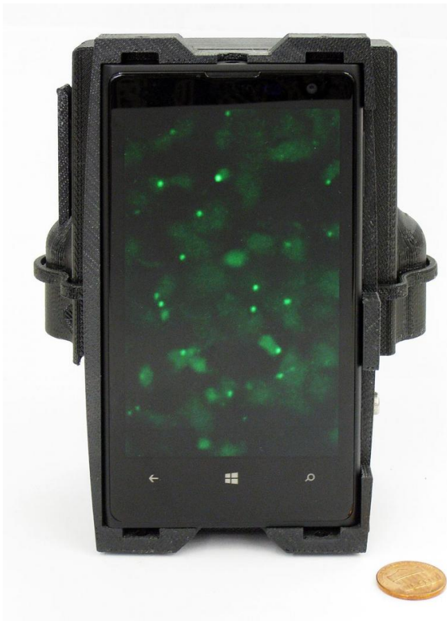
Device using fluorescent image mode. Credit: UCLA, Stockholm University and Uppsala University
