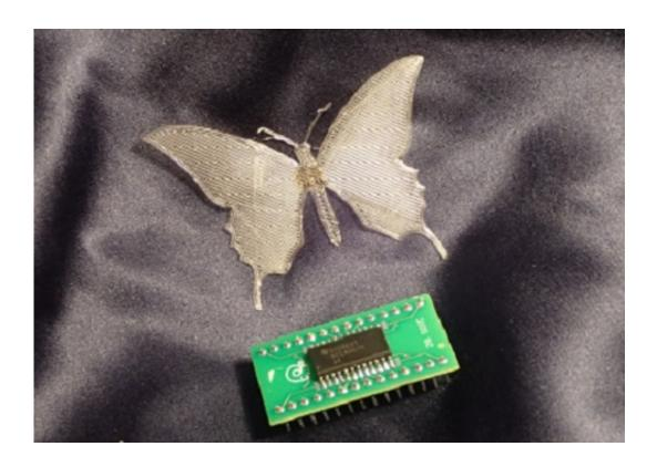
Pressure-sensitive 'e-stickers' contain all the functionality of traditional silicon circuits but can be fabricated into complex, flexible shapes such as butterflies. Credit: © 2016 KAUST
