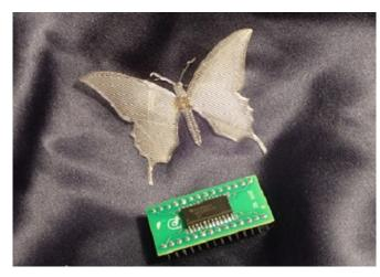
Pressure-sensitive 'e-stickers' contain all the functionality of traditional silicon circuits but can be fabricated into complex, flexible shapes such as butterflies. Credit: © 2016 KAUST
