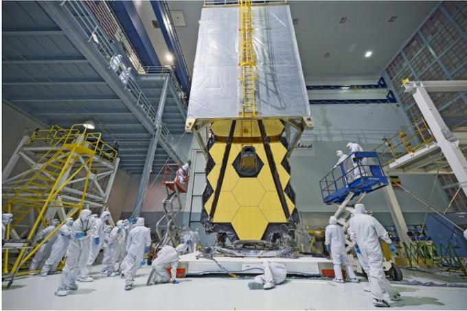
The 6.5 meter diameter 'golden' primary mirror is comprised of 18 hexagonal segments – looking honeycomb-like in appearance.
