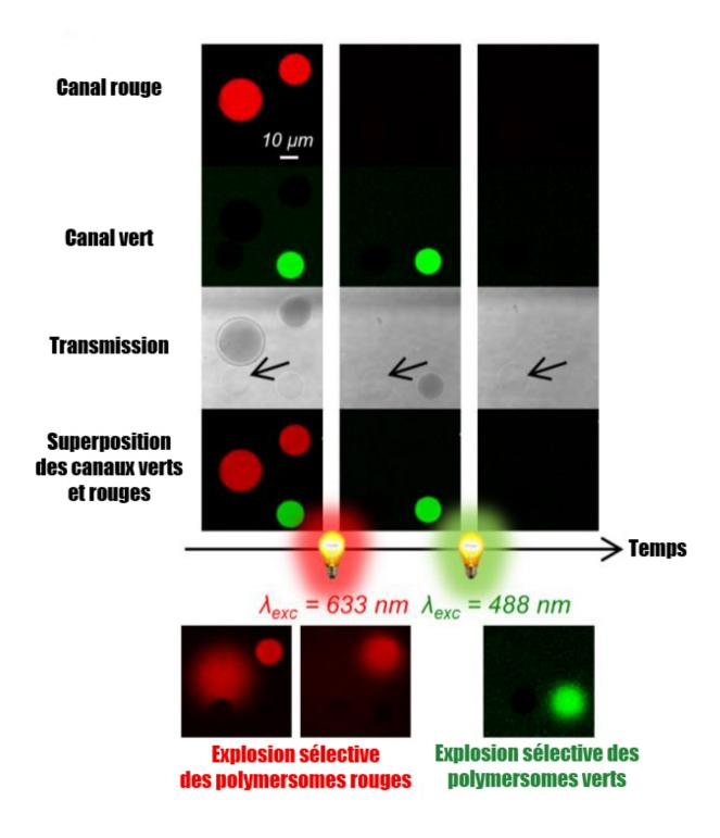
Confocal microscope observations of three types of vesicles. In red, methylene blue-loaded vesicles; in green, calcein-loaded vesicles. Sucrose-loaded vesicles are indicated by an arrow. Laser irradiation of 633 nm then 488 nm ruptures the red and green vesicles in succession. The other vesicle remains intact. Credit:
