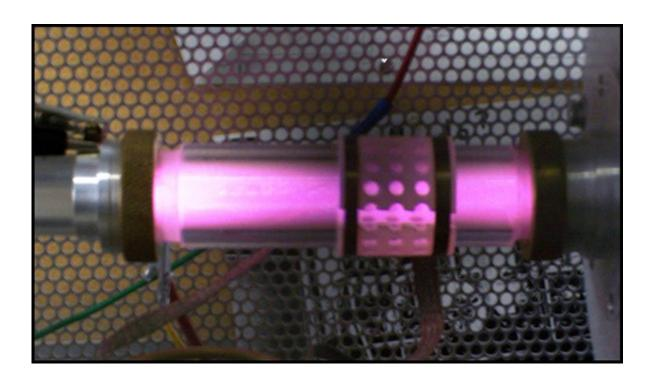
Scientists used this radio frequency discharge source to measure the extremely low abundance of <sup>3</sup>He in samples of purified helium, the gas used in precision neutron lifetime experiments. Credit: US Department of Energy
