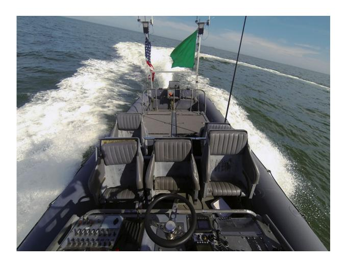
An unmanned rigid-hull inflatable boat operates autonomously during an Office of Naval Research (ONR)-sponsored demonstration of swarmboat technology held at Joint Expeditionary Base Little Creek-Fort Story. During the demonstration four boats, using an ONR-sponsored system called CARACaS (Control Architecture for Robotic Agent Command Sensing), operated autonomously during various scenarios designed to identify, trail or track a target
