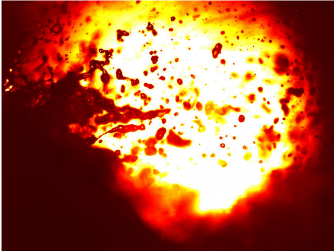
False color image of spray droplets being ejected from a breaking wave (left side of frame), taken in the laboratory. The droplets are moving from left to right in the air and the biggest drops are about 1-2 mm across. Credit: UM Rosenstiel School of Marine and Atmospheric Science - SUSTAIN laboratory, Ortiz-Suslow
