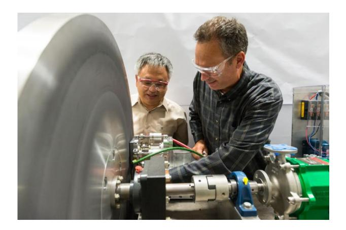
Argonne high-energy physicist Wei Gai and engineer Scott Doran work on a newly developed positron target that could help provide a key component for the proposed International Linear Collider. Credit: Wes Agresta/Argonne National Laboratory
