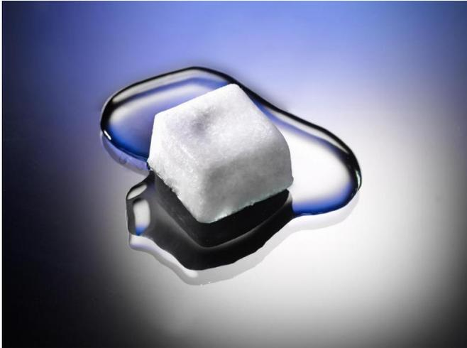
The PCM cube maintains a temperature of 21 degrees Celsius until it is completely melted. Credit: Fraunhofer ICT
