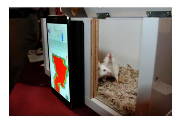
In this Thursday, Nov. 17, 2016, photo, a Walabot, a handheld 3-D imaging system by Vayyar, senses two mice during a demonstration at Pepcom, in New York. Walabot's sensor technology can look through walls to detect structural foundations, track a person's location and vital signs as they move through a Smart Home, measure the speed of a fast-moving ball, and help drones and cars avoid collisions. (AP Photo/Richard Drew)
