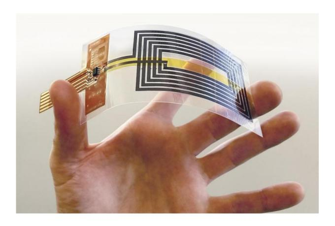
Flexible NFC Antenna. Credit: Graphene Flagship
