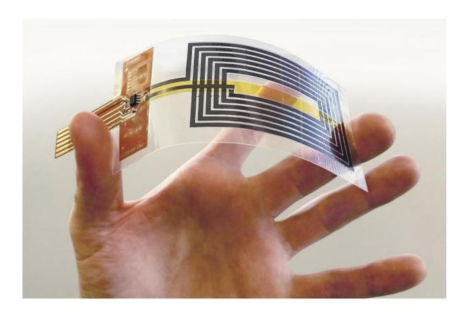
Flexible NFC Antenna. Credit: Graphene Flagship
