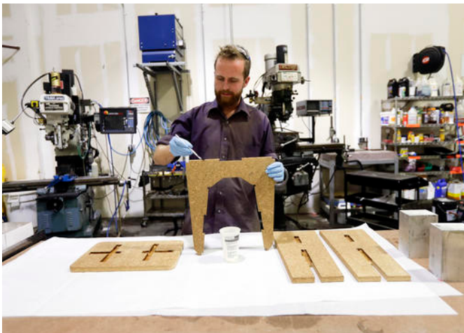
In this Tuesday, Sept. 27, 2016 photo, prototype engineer Kenneth Lush assembles a stool at Ecovative Design in Green Island, N.Y. Ecovative Design is a business staking its growth on mycelium, the thread-like "roots" of mushrooms. The mycelium grows around small pieces of stalks and stems to create a bound-together material that can be molded into soft packaging for glassware or pressed into the boards used for the footstools they recently began selling. (AP Photo/Mike Groll)
