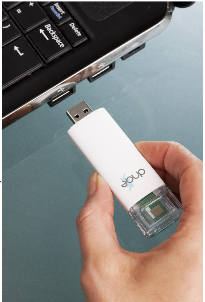
USB stick that tests for HIV. Credit: Imperial College London / DNA Electronics
