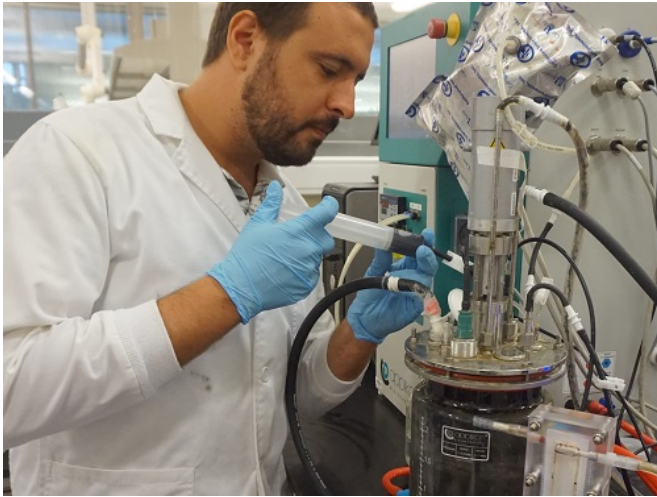
Moustapha Harb collects a water sample from the anaerobic membrane bioreactor. Credit: KAUST
