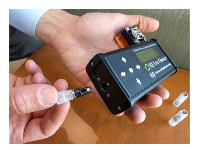
A thermophoretic sampler first developed at Colorado State University will spend 32 days at the International Space Station detecting dust particles for later analysis. Credit: Anne Manning/Colorado State University
