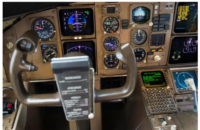
Data Communications Data Comm technology, lower right, is seen in the cockpit of an UPS Boeing 767-300F aircraft at Dulles International Airport Air Traffic Control Tower in Sterling, Va., Tuesday, Sept. 27, 2016. Data Comm gives air traffic controllers and pilots the ability to transmit flight plans, clearances, instructions, advisories,
