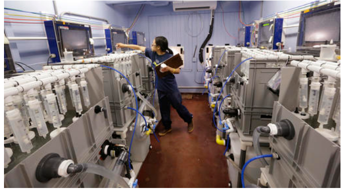
Audrey Djunaedi, a lab technician with NOAA's Northwest Fisheries Science Center, places containers holding individual Dungeness crab larvae into tanks where the crabs are exposed to simulated current conditions as well as what can be expected in the future as the seas absorb more carbon dioxide, in Mukilteo, Wash., on July 26, 2016. Not all species of crabs are affected by ocean acidification in the same way. And the broad range of habitats that Dungeness crabs occupies along the West Coast gives him hope that they can persist and do well in some environments even if they don't in others. (AP Photo/Elaine Thompson)
