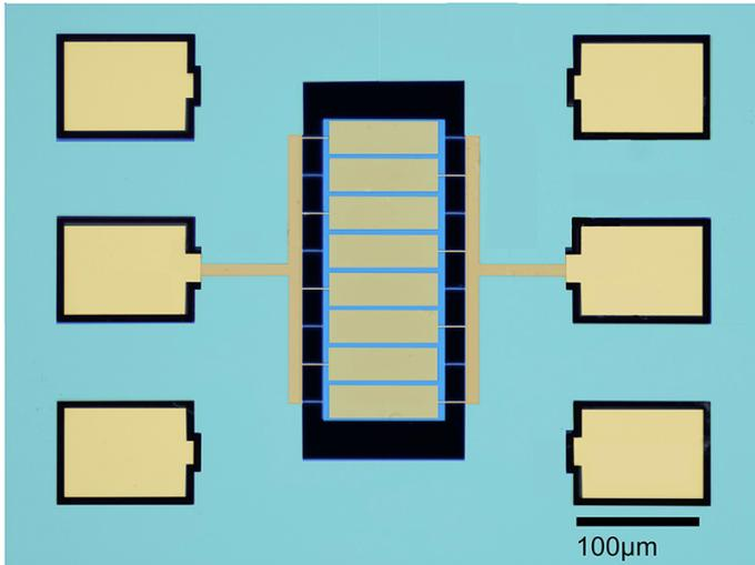
A wireless micromachine. The miniature sandwich of gold and aluminum nitride is 100 micrometers across—a little wider than the width of a human hair. Credit: Boston University
