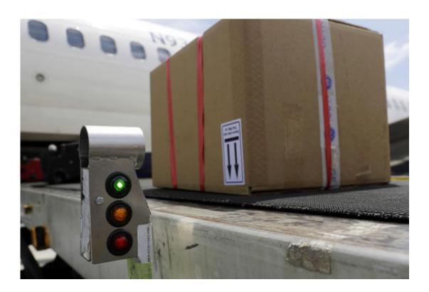
In this July 12, 2016, photo, a scanner displays a green light as it detects an RFID-
