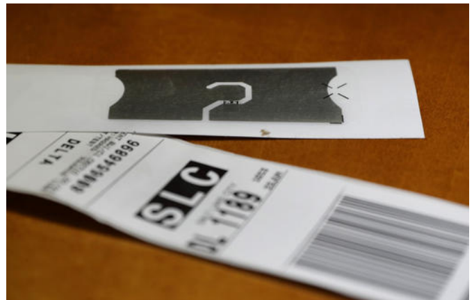
This July 12, 2016, photo, shows the inside of a sample RFID-enabled Delta Air Lines baggage tag, at top, at Baltimore-Washington International Thurgood Marshall Airport in Linthicum, Md. Delta Air Lines is rolling out new technology to better track bags throughout its system. (AP Photo/Patrick Semansky)
