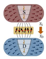
In the proposed experiment, two energy reservoirs (S and D) made of trapped ions transport energy quanta to each other by coupling to the spins in a quantum magnet placed between them. Credit: Alejandro Bermudez and Tobias Schaetz, *New Journal of Physics*. CC-BY-3.0
