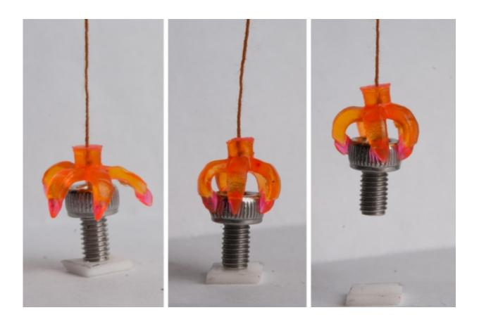
In this series, a 3-D printed multimaterial shape-memory minigripper, consisting of shape-memory hinges and adaptive touching tips, grasps a cap screw. Credit: Qi (Kevin) Ge
