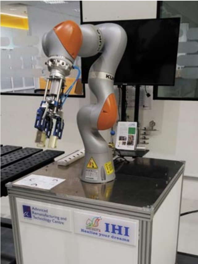
The KUKA LBR iiwa 7 R800 collaborative robot assists with quick shop-floor automation for the manufacturing industry. Credit: A*STAR Advanced Remanufacturing and Technology Centre
