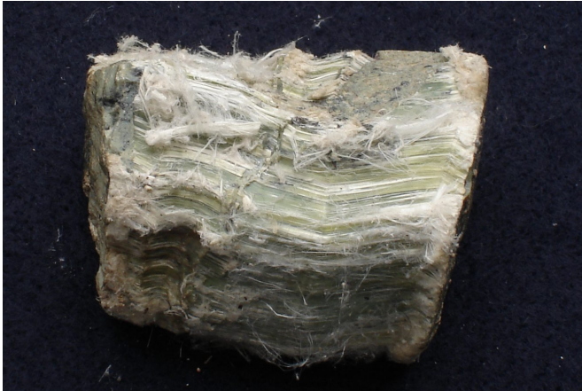
Chrysotile is one of the six types of asbestos. Credit: Eurico Zimbres/WikiMedia
