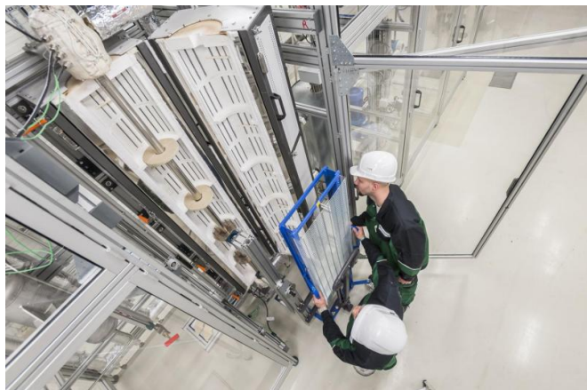
Pilot plants for the chemical conversion and processing of fuels and fuel additives: High-pressure flow tube reactor. Credit: Fraunhofer-Gesellschaft
