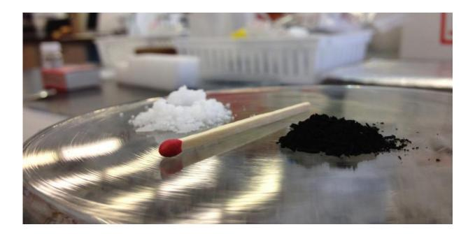
Preparing conducting carbon nanospheres that operate as qubits at room temperature (right) by burning naphthalene (left). Credit: Dr Mohammad Choucair, Author provided
