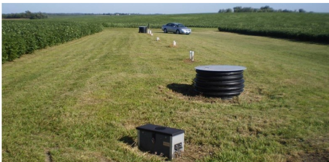
Monitoring wells above an installed bioreactor on a research farm in Iowa. Credit: Laura Christianson.
