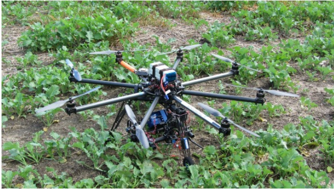
The eight-rotor octocopter mounted with a multi-sensor sensor camera is diagnosing stress levels in plants. Credit: Science Network WA
