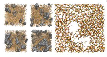
In modeling new protective materials, the researchers introduced sacrificial molecules (shown in grey) in the four-frame simulation on the left. These molecules can be removed after the material is made, leaving behind tiny pores (visible in the larger frame on the right) that make the material more durable to expansion and contraction. Credit: Dauskardt Group
