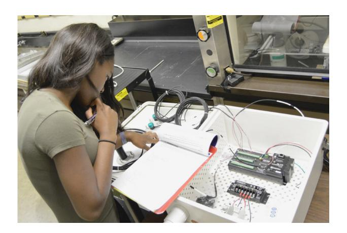
Energy engineering undergraduate student Worlasie Djameh inspects the wiring configuration of the All-Seeing Eye device prior to installation. The device was created to collect more baseline information about sunlight, which can be used to inform a variety of industries. Credit: Penn State
