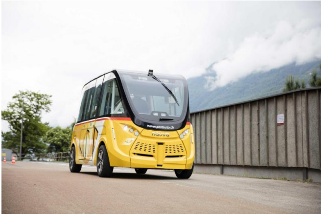
Autonomous shuttles will carry up to 11 passengers at a time. Credit: Car Postal
