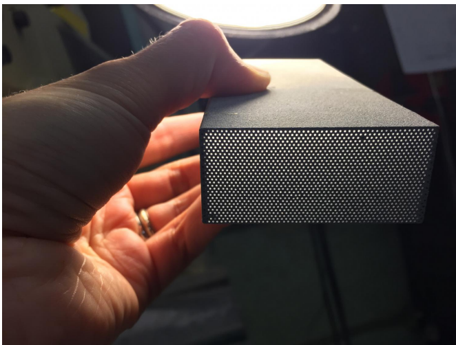
A closeup of the scintillating fibers traversing one of the tungsten bricks designed to track electrons and photons in the sPHENIX electromagnetic calorimeter. (Photo credit: Anne Sickles)
