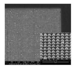
The focused ion beam fabricated trilayer metasurface within the inset shows rounded features in the upper 2-D gold square periodic surface. Credit: University of Bristol
