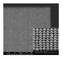
The focused ion beam fabricated trilayer metasurface within the inset shows rounded features in the upper 2-D gold square periodic surface. Credit: University of Bristol
