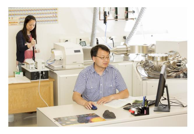
Co-authors Yan Hu (l) and Fang-Zhen Teng with the MC-ICP-MS machine (right) that turns basalt into a plasma, in which electrons are separated from each atom's nucleus, to discover tiny variations in the rock's chemical makeup. Credit: Dennis Wise/University of Washington
