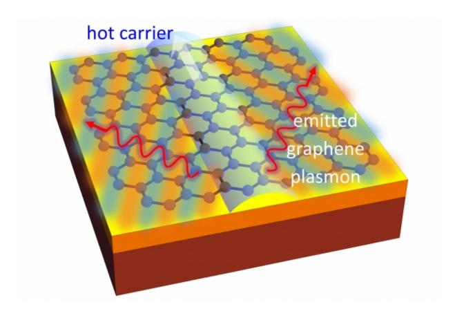
This illustration depicts the process of light emission from a sheet of graphene, which is represented as the blue lattice on the top surface of a carrier material. The light-colored arrow moving upwards at the center depicts a fast-moving electron. Because the electron is moving faster than light itself, it generates a shock wave, which spews out plasmons, shown as red squiggly lines, in two directions. Credit: Massachusetts Institute of Technology
