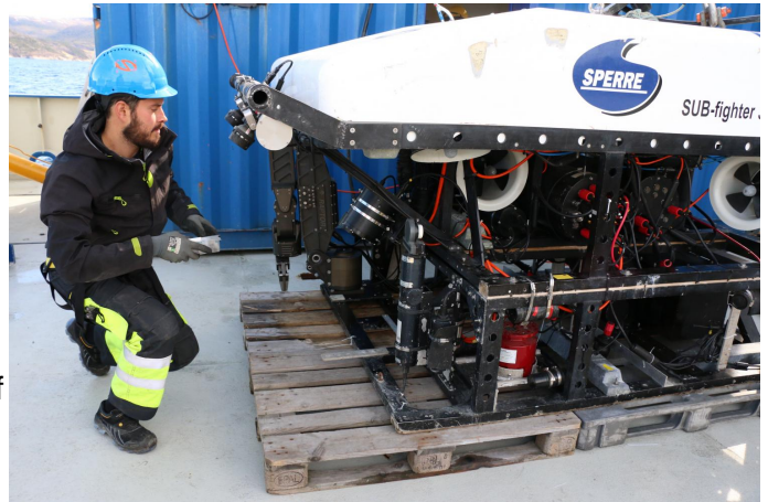
Pedro Roberto De La Torre Olazabal examines the HD camera mounted on the two-tonne ROV that will help researchers explore the bottom of Trondheim fjord. Credit: Nancy Bazilchuk, NTNU
