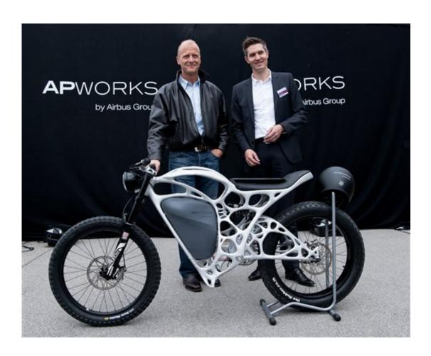
The CEO of Airbus, Tom Enders, left, and the head of APWorks, Joachim Zettler, present the first 3D printed electric motorcycle in Ottobrunn, Germany, Friday May 20, 2016. The motorcycle was made of metal powder by using lasermelting technology. The bike only weighs 35 kilos. (Sven Hoppe/dpa via AP)
