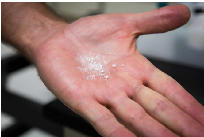
Nano-scale diamondoid crystals, seen above, are derived from petroleum. They have potential for applications in energy, electronics, and molecular imaging. Credit: Nick Melosh
