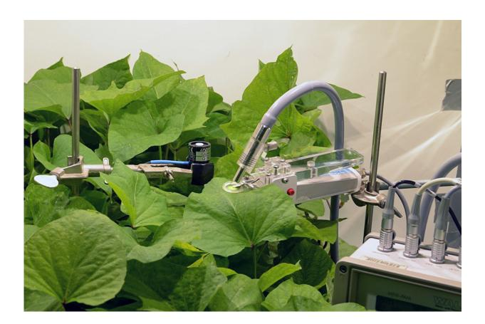
A sweetpotato crop is shown in the biofeedback system. Chlorophyll fluorescence measurements are taken on the plant on the right side to determine how efficiently the plant uses the light provided by LEDs. LED light levels are automatically adjusted to maintain specific levels of physiological activity. Credit: Photo courtesy Michael T. Martin.
