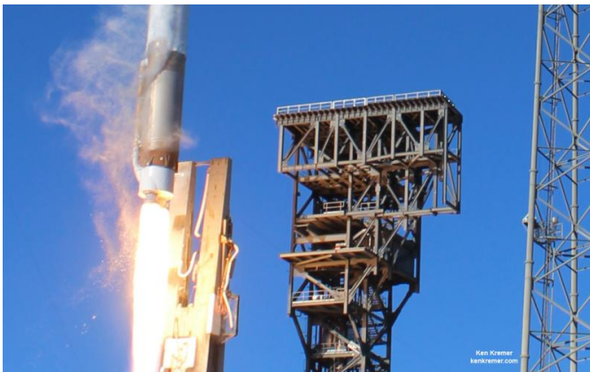
Up close view of dual nozzle RD-180 first stage engines firing during blastoff of United Launch Alliance (ULA) Atlas V rocket carrying the GPS IIF-12 mission on Feb. 5, 2016 from Space Launch Complex 41 on Cape Canaveral Air Force Station, Fla. Credit: Ken Kremer/kenkremer.com
