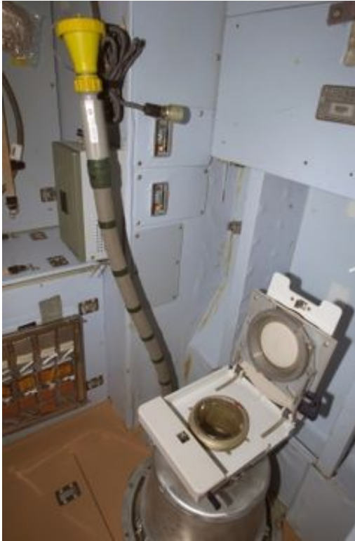
Toilet at the International Space Station. Credit: NASA
