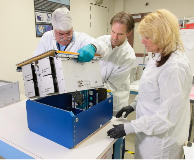
Under the direction of the International Space Station Utilization Office and the Space Biology Project, NASA's Rodent Research Hardware System was developed and built at NASA's Ames Research Center to provide a research platform for long-duration rodent studies in space. Credit: NASA
