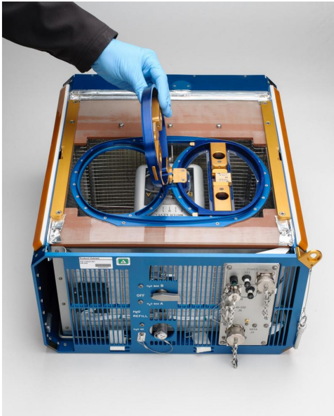
NASA's Rodent Habitat, shown here with one of the two access doors open, provides long-term housing for rodents aboard the International Space Station. Credit: NASA/Dominic Hart
