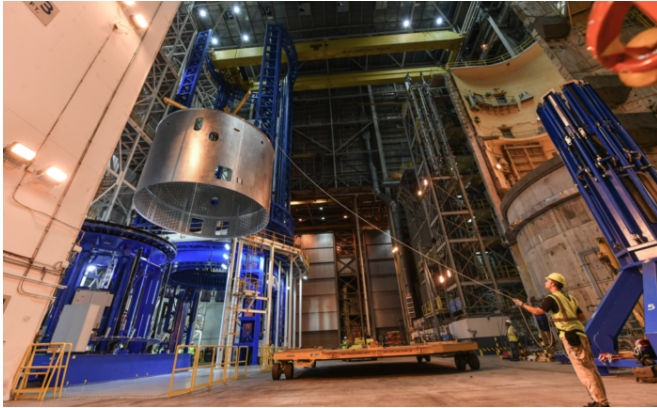
Space Launch System (SLS) core stage engine section finishes welding at the Vertical Assembly Center at NASA's Michoud Assembly Facility in New Orleans for maiden flight of SLS rocket. Credit: NASA
