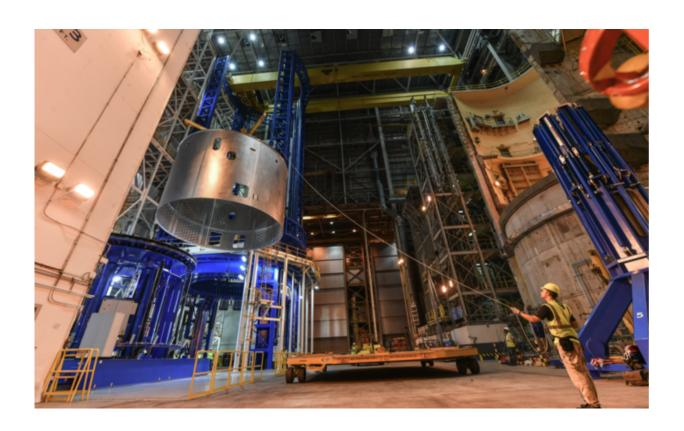
Space Launch System (SLS) core stage engine section finishes welding at the Vertical Assembly Center at NASA's Michoud Assembly Facility in New Orleans for maiden flight of SLS rocket. Credit: NASA
