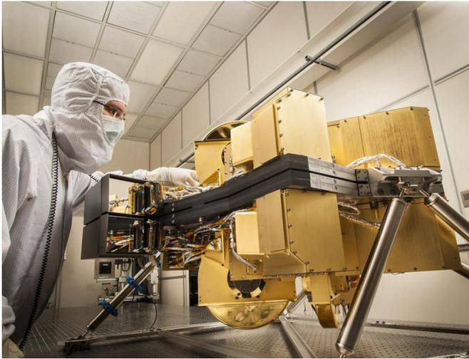
NIRCам (left) beat requirements during final cryogenic testing with the Integrated Science Instrument Module for the James Webb Space Telescope. The module recently completed testing at NASA's Goddard Space Flight Center.
