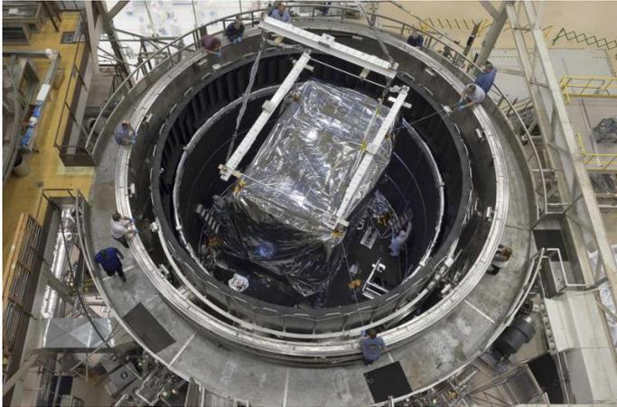
NIRCam beat requirements during final cryogenic testing with the Integrated Science Instrument Module for the James Webb Space Telescope. The module recently completed testing at NASA's Goddard Space Flight Center. Credit: NASA
