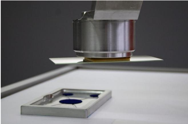
New robotic gripping surface for sensitive and heavy devices.
