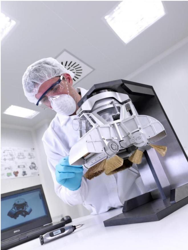
Designed and built by Added Value Solutions of Spain, the machine automatically detects the distance between the brushes and the surface to adapt as necessary, collect the dust, and direct it into a hermetically sealed box for storage and analysis.
