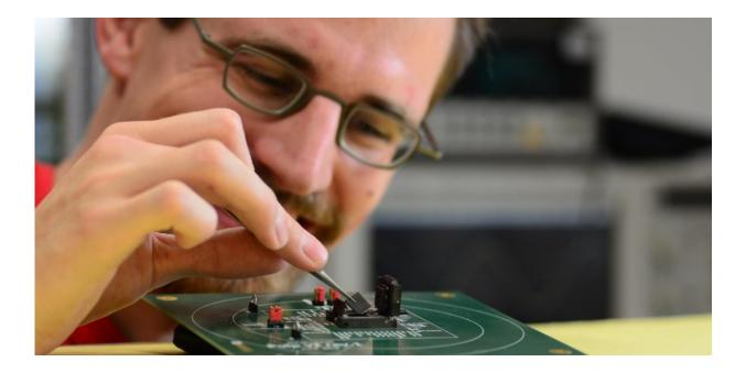
An ETH scientist uses tweezers to mount a PULP microprocessor on to a test board for measurement. Credit: ETH Zurich / Frank K. Gurkaynak
