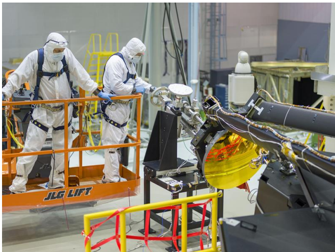
In this photo, engineers are seen installing the secondary mirror onto the telescope. Credit: NASA/Chris Gunn
