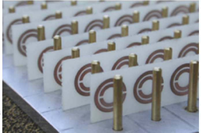
An early metamaterial using repeating elements of copper split-rings and copper wires. Credit: D. R. Smith et al., Left-handed Metamaterials, in Photonic Crystals and Light Localization, ed. C. M. Soukoulis (Kluwer, Netherlands, 2000)., CC BY-ND
